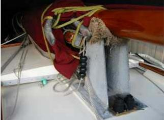
Lash the mass of ropes lying in the forward part of the cockpit to the mast and scoop up the ones lying in the rear with the sheet, wrapping it around the mast and starting with the stern end. Pick up the front ends of the sheet; hold them on top of the mast with one hand whilst stuffing the ropes into the belly. When they are all in (easier done than described) lash the whole mess closed. The cockpit is then clear and tidy, and access to the cabin is possible.
