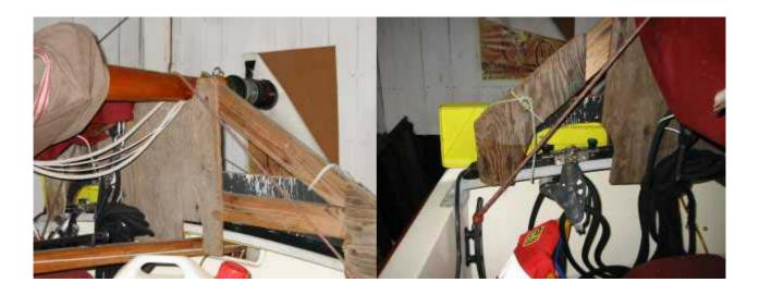
Pull the jib sheets in tight, close up the cabin, fasten lighting board and cable, and strap the boat down to the trailer.
